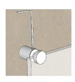
4 Slide the grips/panel onto the anchors. Tighten the outside M4 set screw once all grips are seated flush against the anchors.
